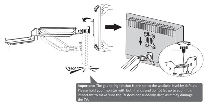
**STEP 7:** Adjust the gas spring tension to your personal preference using the 6 mm Allen Key (G). You may also adjust the tilt tension using 6 mm Allen Key (G).
