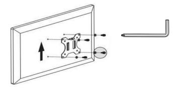
**STEP 6:** Put each assembled TV with the attached VESA Plate (B) onto each Arm Assembly (A). Ensure stability and then insert the Top Bolt (E) to hold each TV in place.
