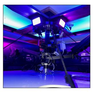
Attach the bungee cords to the top corners of your Light / Bungee Bracket. Make sure you have a helper as you lift up the base up and center the base flange onto the pole. Attach the bungee cords to the corner eye pads of the base and evenly tighten the flange screws to securely level and attach the base onto to the pole.
