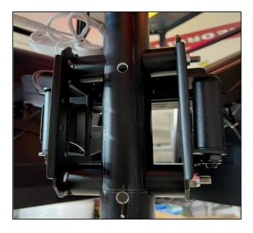
Grab your 4 TV mounts and the Quad Mount Pole Hardware consisting of a 4 long bolts, 8 washers, 8 saddle spacers, and 4 nuts. You're going to attach two mounts to the pole using 2 bolts, 4 washers, 4 saddle spacers and 2 nuts. Then repeat the steps to firmly attach the other two mounts.
