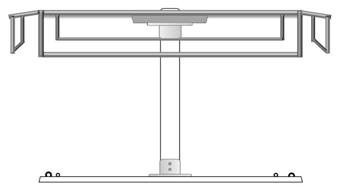
EITHER REMOVE THE FRAME WHILE INSTALLING THE TVs OR RAISE AND TIGHTEN THE FRAME UP AS HIGH AS YOU CAN SO IT IS OUT OF THE WAY DURING INSTALLATION OF THE TVs.
