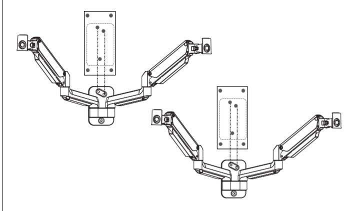
**STEP 5:** Attach both Dual Arm Assemblies (A) to the Pole (D) about 1" above the silver flange using the remaining 4 long bolts, lock washer and nut. Tighten the 4 bolts equally and securely so that the brackets permanently grip the pole and to prevent the mounts from sliding down the pole. Be careful not to overtighten or you may snap the bolts.
