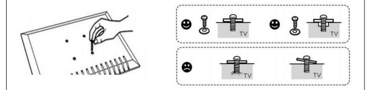
Once you find the correct screws, attach the VESA Plate (B) to the back of each TV using 4 washers, 4 screws and the screwdriver side of the included 6 mm Allen Key (G).
