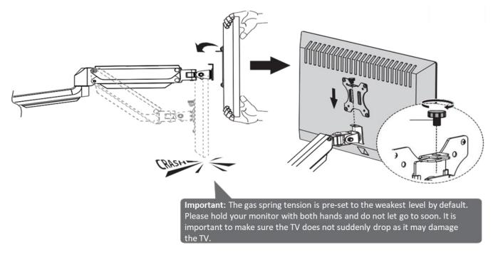
**STEP 8:** Adjust the gas spring tension to your personal preference using the 6 mm Allen Key (G). You may also adjust the tilt tension using 6 mm Allen Key (G).
