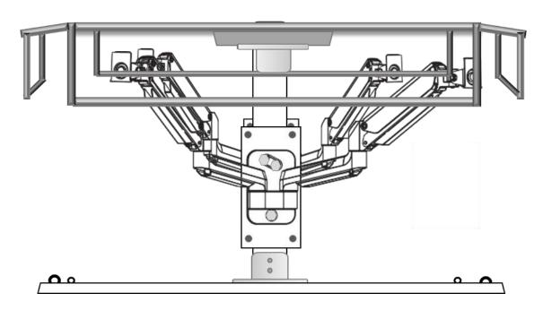
STEP 6: Attach the VESA Plates (B) to the back of each TV using the appropriate sized screws.
