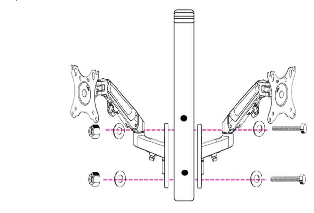
**STEP 4:** Mount the TVs. Locate the correct set of screws for your TVs. You may find it easier to hang the TVs if you first attach the top two screws into the back of the TV and then set your TV onto the mounting plate.
