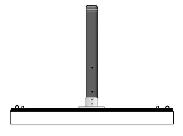
**STEP 2:** Assemble the Quad TV Mounting System using the appropriate hardware.
