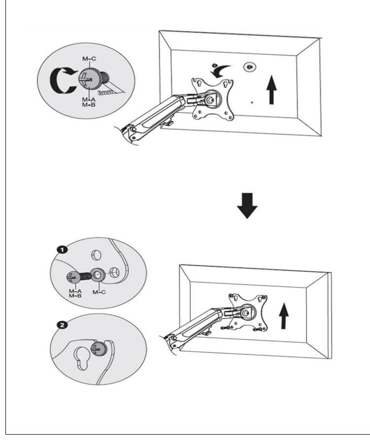
**STEP 5:** Adjust the gas spring tension to your personal preference using the Allen Key (G). You should be able to physically lower the TVs and position them onto of the foam on the base.
